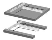
An uneven foundation might cause malfunction or jammed panels. Liability is excluded for damage caused by installation on an uneven surface.
