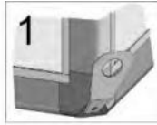
Variation 1 Crane strap on the corner bracket
