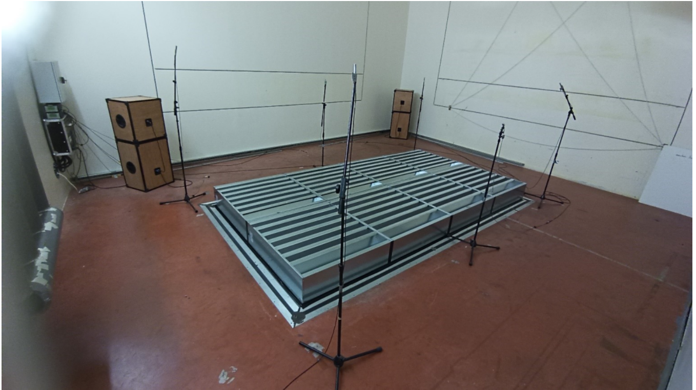
Figure 4 – Sample G28 set up on the reverberant room floor.
