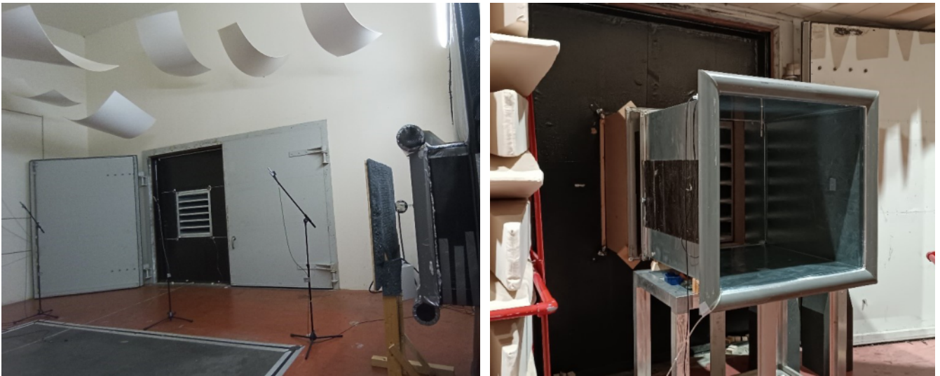
Figure 2 - Installation of the sample as seen from the reverberant room and from the semi-anechoic room installed in the upstream section of guide.
