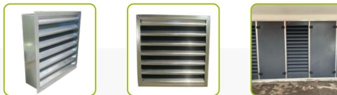
As standard, the Solflex acoustic louvres are made of galvanized or powder-coated sheet metal in RAL colors. Depending on the insulation required, the depth of the blinds can be selected from **4 available dimensions** (200, 300, 400 and 600mm depth). The width is arbitrary possible for 100mm from 300 to 2.500mm. The height is arbitrary possible, each 150mm from 450 to 2.250mm.
